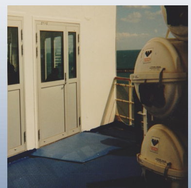
An elevated (heated) access ramp with the Conficomp technology, onboard Stena Danica.
