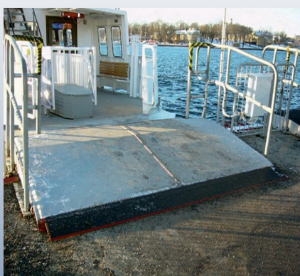
Access ramp with integrated heating function on a small passenger ferry in the Baltic sea.
